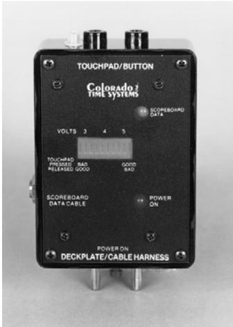
The test meter is a tool to help you quickly troubleshoot a variety of equipment issues with your swim timing system. You can use it to test touchpads, pushbuttons, cable harnesses, deck plates, under-block connection hubs and your timing console's scoreboard output.
