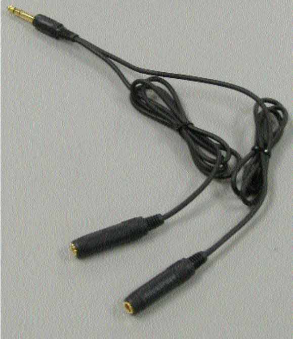
Figure 2-B: Y-adaptor scoreboard data splitter
