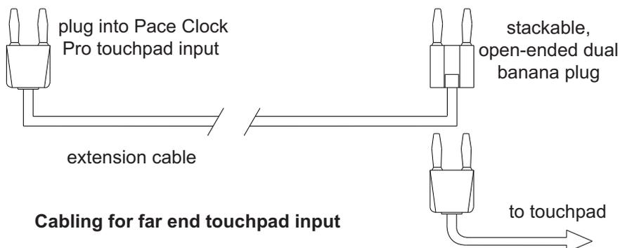
To take input from touchpads at both ends of the pool, plug the touchpad from one end of the pool into either touchpad input on the Pro Pace clock. Plug the touchpad from the other end into the other touchpad input, using an extension cable (CTS SJ series) with a stackable, open-ended dual banana plug.
